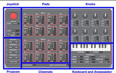
The MPK mini Editor has a straightforward graphical user interface that can be broken down into the following sections:
